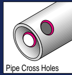
Pipe Cross Holes
